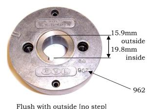
Flush with outside [no step] taper 5 deg
