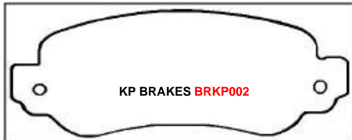
Figure 7 [No Threaded Mounting Holes] 14.5 Thick
