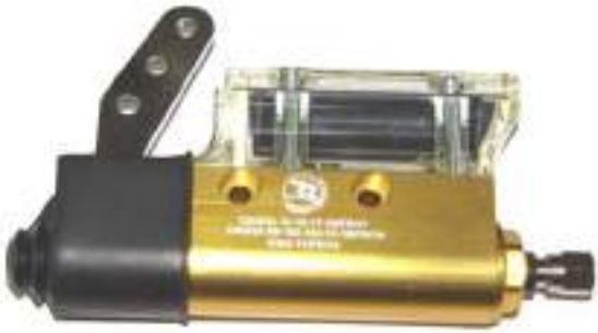
Hydraulic Brake Master Cylinder full compensation reservoir type 7/8" Bore Diameter 35mm c to c x 6mm mounting part number BRRRK225XGOLD
