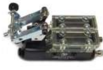
M/CYL OPTION 2 X Master Cylinder Plus Brake Bias assembly
