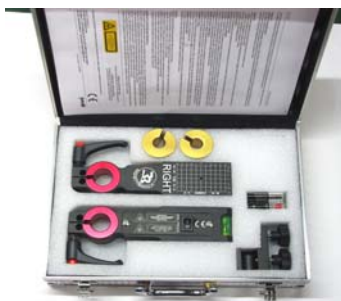
RIGHETTI RIDOLFI LASER ALIGNMENT KIT SUITS 17mm & 20mm AXLE SHAFTS
