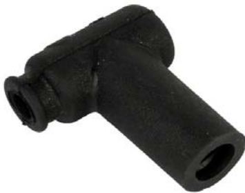
5 ohm RESISTOR CAP same as LATE YAMAHA part number SP013
